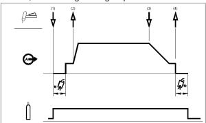
Press and hold the TIG torch trigger to start the sequence. The machine will open the gas valve to start the flow of the shielding gas. After the preflow time, to purge air from the torch hose, the output of the machine is turned ON. At this time the arc is started according to the selected welding mode. After the arc is started the output current will be at the Start current. This condition can be maintained as long as necessary.
