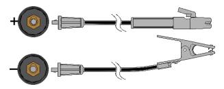
Connect the electrode cable to the (+) terminal and the work clamp to the (-) terminal. Insert the connector with the key lining up with the keyway and rotate approximately ½ turn clockwise. Do not over tighten.
