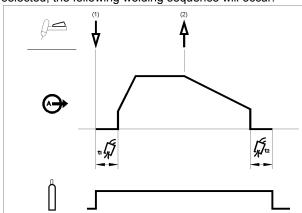
Press and hold the TIG torch trigger to start the sequence. The machine will open the gas valve to start the flow of the shielding gas. After the preflow time, to purge air from the torch hose, the output of the machine is turned ON. At this time the arc is started according to the selected welding mode. After the arc is started the output current will be increased at a controlled rate, or upslope time, until the Welding current is reached.
