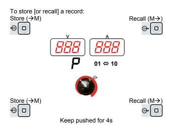
The Memory pushbuttons are disabled during welding.
