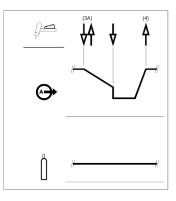
Welding current, like in step 4, to continue welding. When the main part of the weld is complete go to step 3.
