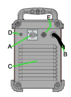
ON only for the startup time (few seconds). The fan will start with welding operations and will continue to run whenever the Machine is welding. If the Machine doesn't weld for more than 10minutes, it will go in Green Mode.
