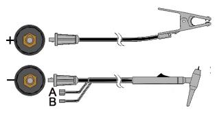
Connect the torch cable to the (-) terminal of the machine and the work clamp to the (+) terminal. Insert the connector with the key lining up with the keyway and rotate approximately ¼ turn clockwise. Do not over tighten.
