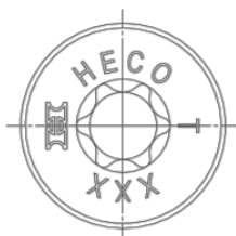
Head markings for d = 6.0 to 10.0 of types: flat countersunk head. Specified type without lettering possible too.
